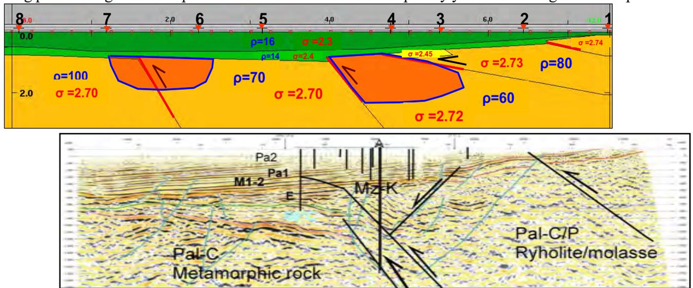
Figure 2: Example of a mult-physic interpretation of electromagnetics to geothermal applications. The top section shows the gravity and electromagnetics (magnetotelluric) interpreted model where low rock density and low resistivity coincide in the anomaly in the center. The bottom shows further integration results with the reflection seismic and the drill location in the center that produces in the first days already 4 MW geothermal power (modified after Yu et al., 2009).
