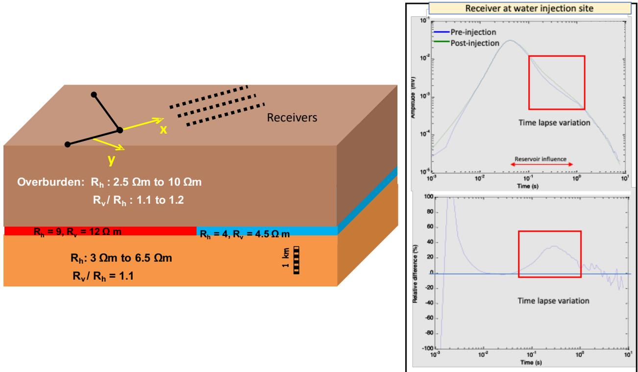
Figure 4: EOR model with anisotropic resistivities and real data CSEM time lapse data response (3 days of water-flooding).
