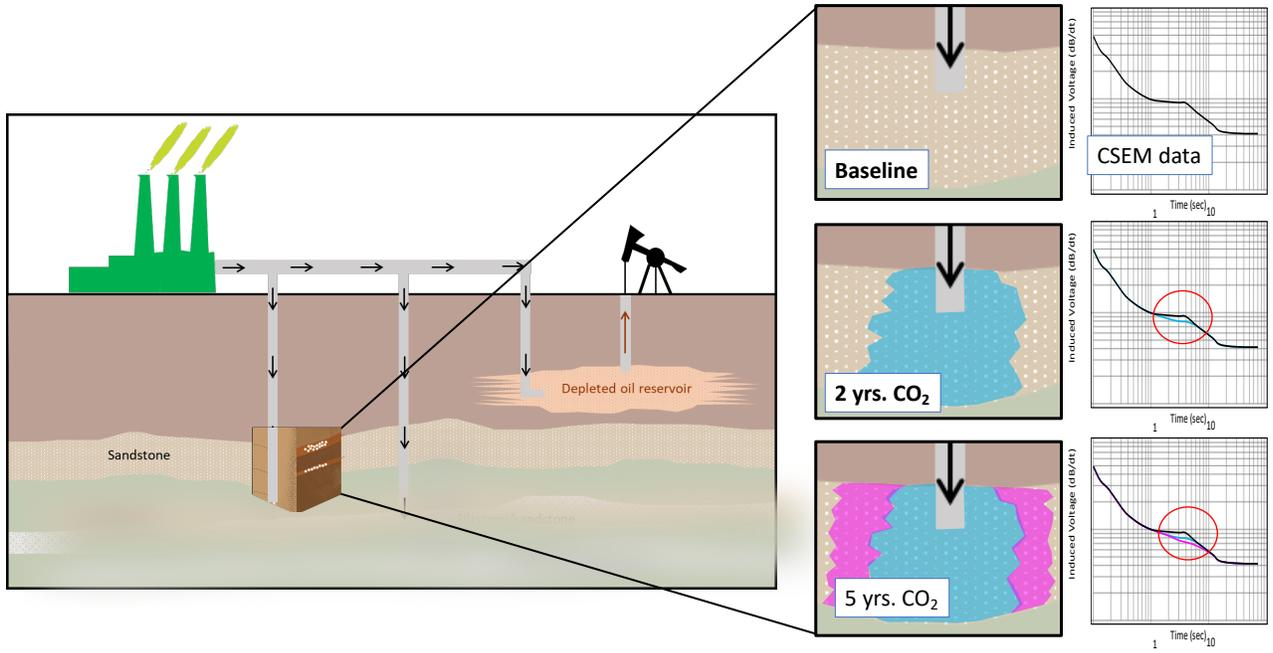
Figure 3: CO<sub>2</sub> Earth model, reservoir model, and CSEM data response curve for different time steps after injecting CO<sub>2</sub> into the reservoir.
