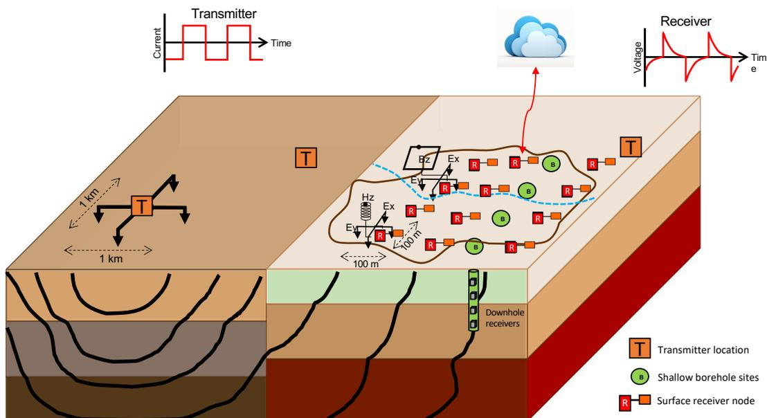
**Figure 1: Controlled Source EM survey layout showing transmitter, receivers, and shallow borehole sensors. Each sensor can have multi-components in electric and magnetic fields as well as 3-component seismic sensors. The contour lines represent lines of equal current densities for progressing time.**
